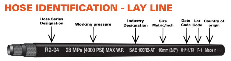
Hose identification is one of the many challenges when replacing a hydraulic assembly. Reference the information printed on the lay line of a hose regardless of the brand. The replacement hose should meet the industry specifications to equal the pressure rating, temperature range, and bend radius of the previous hose.
